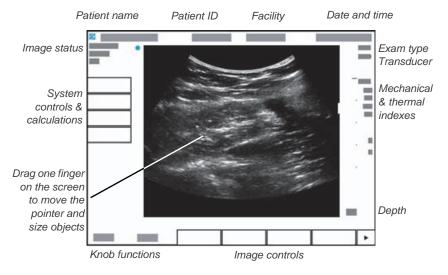
**System controls** The buttons and knobs located below the touchscreen are persistent, but some may be disabled during certain modes or conditions. Controls are lighted when active and dark when disabled. The function of each knob may change depending on the mode or condition.
