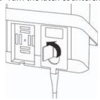
**5** Press the latch down, securing the transducer connector to the system.
