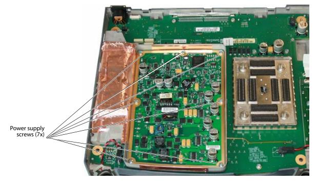
Figure 4.10 Power Supply Screws
