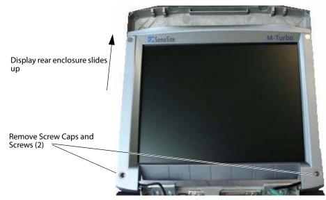
Figure 4.5 Remove Display Back Enclosure
