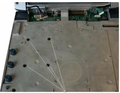
2.5mm Socket Head Cap Screws (4x)
