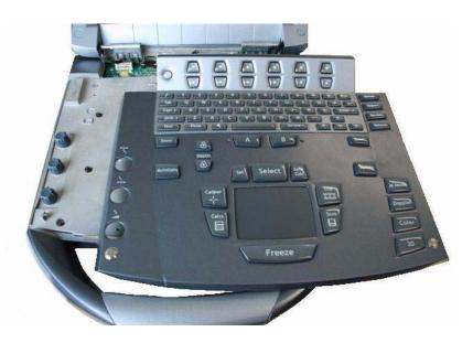
Figure 4.3 Control Panel Removal
